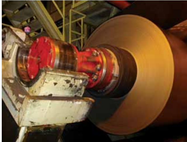
The manufacture of cold rolled annealed steel on the Kawasaki Multipurpose Continuous Annealing Line at USS-POSCO Industries.
